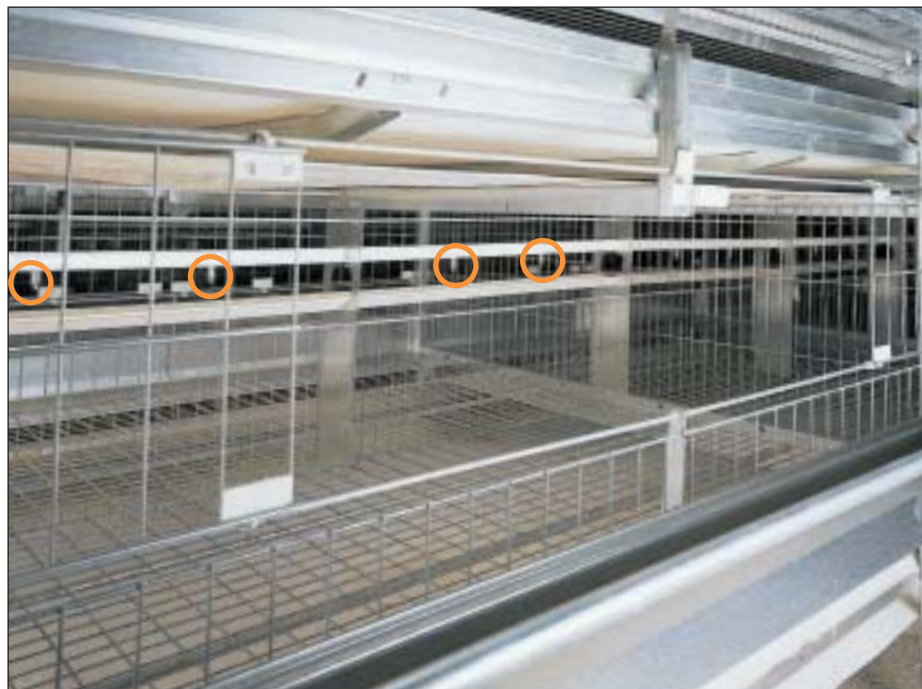
Grow tier UV-S 630 – four stainless steel nipples provide fresh water for the birds
